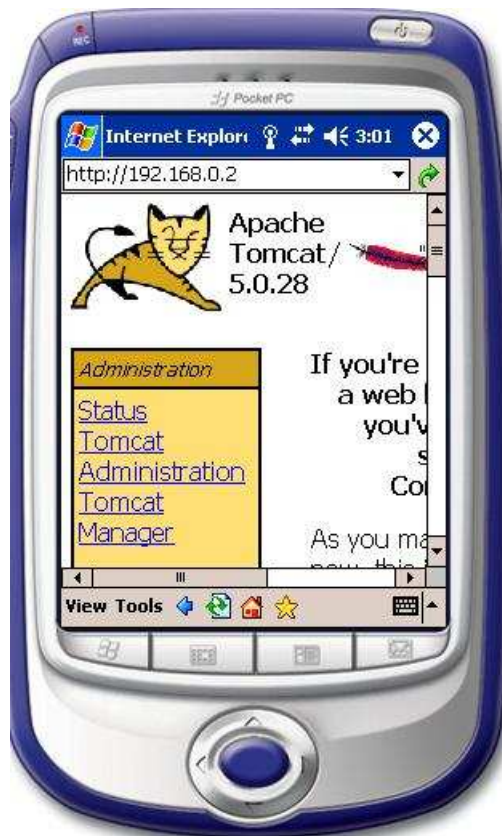
Figure 8.3: The pocket PC can visit the machine with its private IP address
