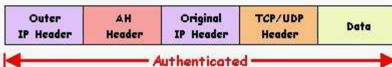
Figure 3.5: IPsec tunnel mode and transport mode.[36]
