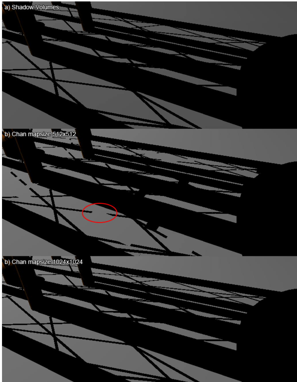
Figure 56: Using too low shadow map size can lead to small or thin objects not to be classified as silhouette pixels, and therefore be wrongly shadowed
