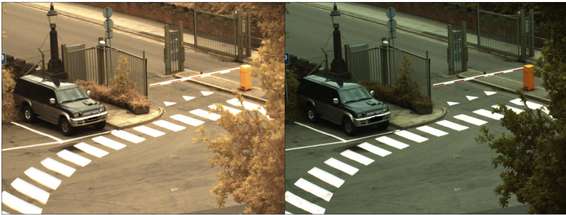
Figure 3.3: Image acquired before (left) and after (right) use of an IR-cut filter (780nm). The CCD is sensitive in the infrared part of the spectrum revealing reddish colors.
