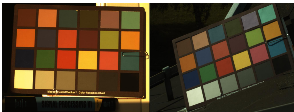
Figure A.1: Images of Macbeth Color Chart with different color temperatures of direct sunlight. (Left): Evening sun - yellowish. (Right): Midday sun - greenish.
