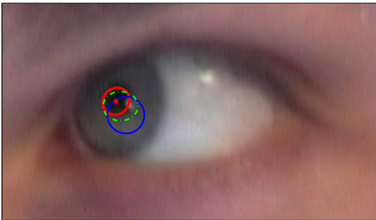
Figure 3: The blue ellipse indicates the starting point of the pupil contour. The template is iteratively deformed by an optimizer; one of the iterations is depicted in green. The red ellipse indicates the resulting estimate of the contour.
