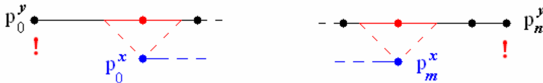
Figure 33. Similarity gap at the beginning and end of paths use to be very frequent, so, path endpoints have to be checked. One (right example) or more (left example) vertices from the same path extremity can fail. Only the vertices from one path (the blue one) would not fail because they have approximation sets on the other path.
