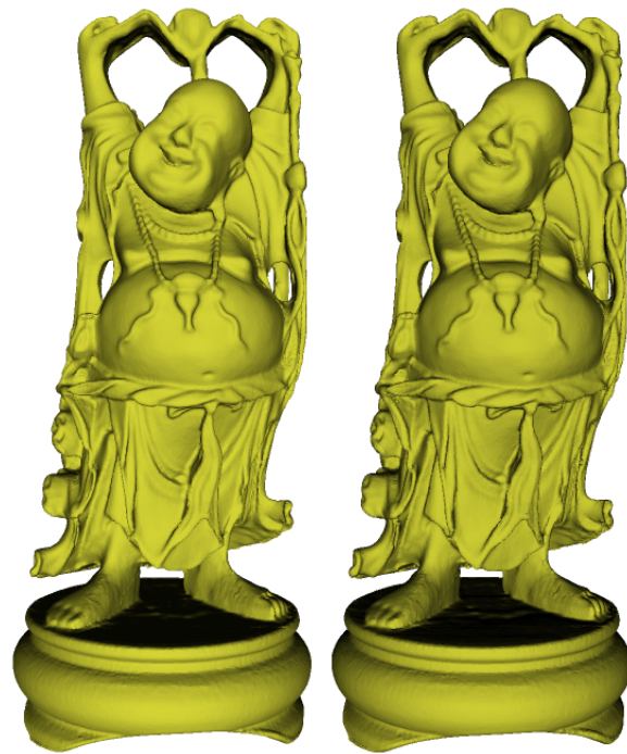
Figure 1: The Happy Buddha model. The original triangle model is on the left, and the point model which consists of 6360009 points (to ensure high fidelity) is shown on the right. Note though that with so many points, the triangle model is actually faster to render (6.7 fps vs. 2.1 fps). Both the mesh model and the point model were rendered using antialiasing.
