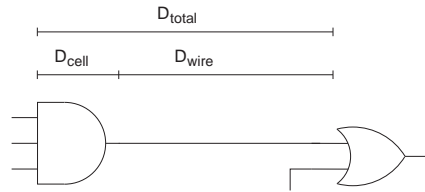
Figure 2.2: Total gate delay split into cell and wire delay.
