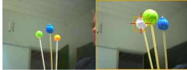
Figure 23: Color weight. The orange colors of a sphere are changed to gray scale representing its weighted value with light as highest weight and dark as low weight. The sphere is close to the camera, to make the weight distribution more clear.
