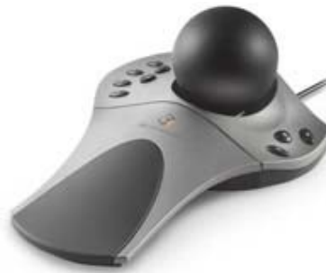
Figure 10: The stationary SpaceBall from Logitech has 6 DOF.
