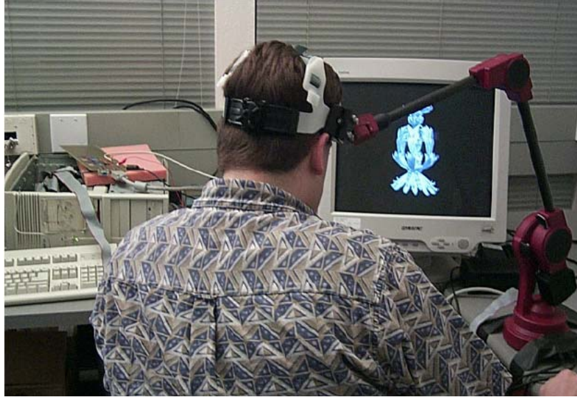
Figure 13: Head-tracking in view dependent rendering or virtual holography.
