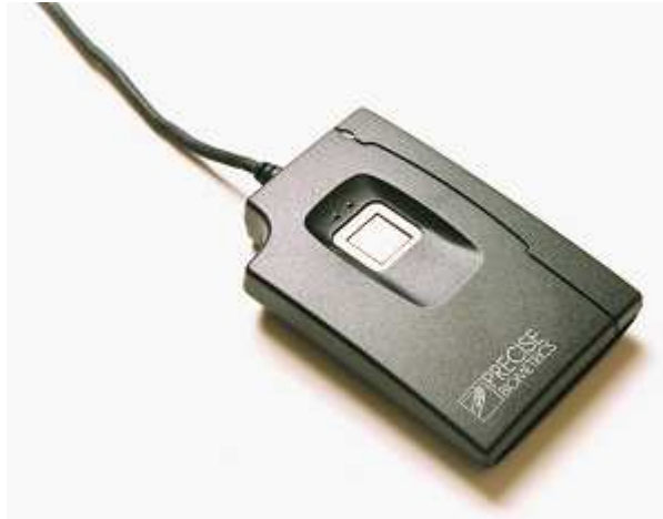
Figure 5.8: Precise 100 MC combined fingerprint and smart card reader. Image courtesy of Precise Biometrics.
