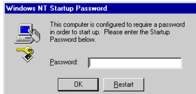
Figure 5.3: Windows NT dialog asking the user to enter the startup password that is required to decrypt the SysKey encrypted SAM database.
