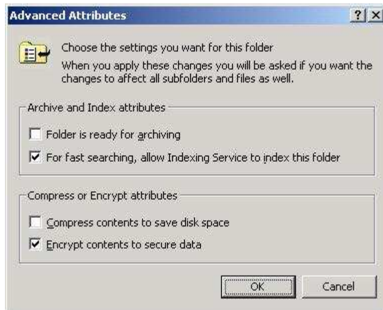
Figure 6.1: The dialog for advanced folder attributes in Windows 2000 includes an encryption check-box.
