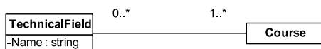
Figure 3.31: Logical model of the TechnicalField class and its association to the Course class.
