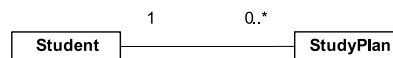
Figure 3.23: Logical model of the association between the Student class and the StudyPlan class.
