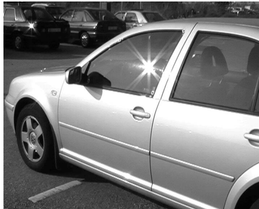
Figure 13.1: Estimating specular surfaces. The specular reflection on the car window gives information on the orientation of the surface normal. An image sequence showing the motion of the specular reflection can be used to estimate the shape of the window. It does not matter that the window is semi-transparent.
