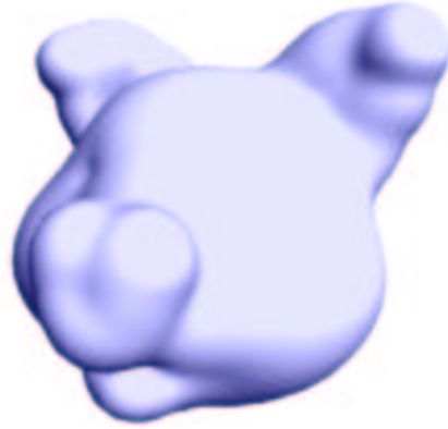
Figure 12.7: This image shows the level 2.2 offset surface of a triangle mesh. The mesh was converted to a distance field using our method, and the offset surface is simply the level 2.2 isosurface of the distance field which was rendered using texture based volume rendering.
