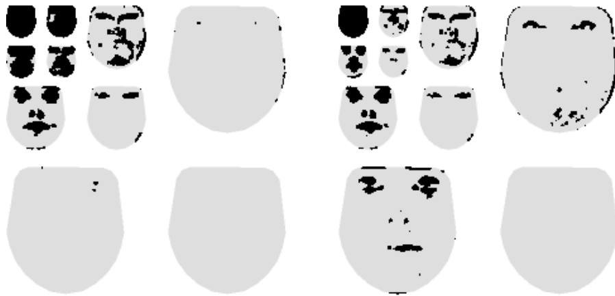
Figure 6. Selected wavelet coefficients for the face training set (CDF, ratio 1:10). The scaling coefficients are shown in the upper left. Left: \|W\|_2 = 1 . Right: \|W\|_2 = 1/\sqrt{2} .
