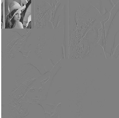
Figure 1. The wavelet coefficients of a two-level octave decomposition using the Haar wavelet.
