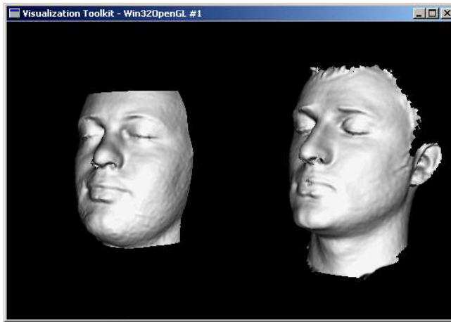
Figure 1: The template shape next to an unregistered face
