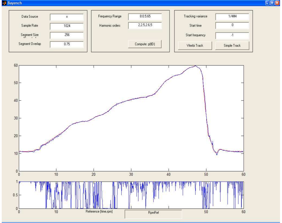
Figure 5.3: Users interface to test program. In the top panel the Bayesian frequency estimator is configured and the tracking parameters set. The frequency range is specified in Matlab TM notation, i.e., it starts at 8 Hz and increases in steps of 0.5 Hz until it ends at 65 Hz. For the simple tracker the regression length, P is specified after the # symbol following the tracking variance. A negative start frequency indicates the tracking should start at the most likely frequency in the first observation. The large graph shows the tracked frequency with a virtually overlapping reference curve. The plot in the bottom panel shows the probability of the tracked frequency in the observations, p(\hat{\omega}_F^{(k)} | \mathbf{d}^{(k)}) .
