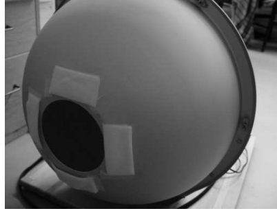
Figure 3.7: Sphere with optimal illumination conditions used to capture the images.
