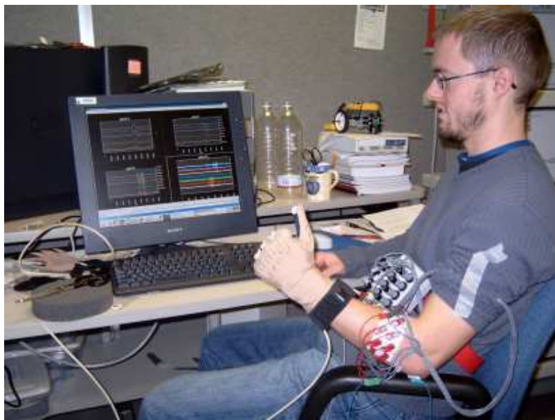
Figure 7.1: Physical setup for acquisition of cyberglove and EMG data
