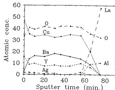
FIG. 4. Sputter Auger profiles for 500 nm thick YBCO film coated with Ag prior to the annealing. The Auger electron probe (10 keV) was focused between the Ag drops. Reliable sputter profiles were difficult to obtain from the LaAlO<sub>3</sub> substrate due to charge pileup.
