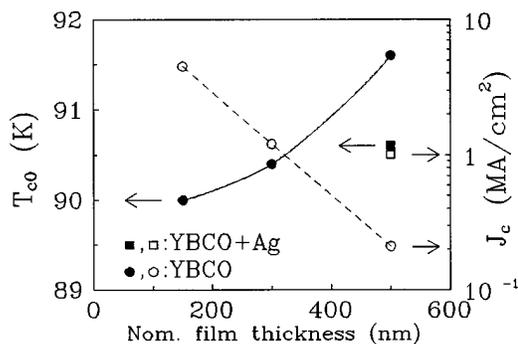
FIG. 1. Zero resistance transition temperature  $T_{c0}$  and critical density  $J_c$  (77 K) vs nominal YBCO film thickness.
