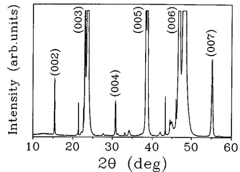
FIG. 3. X-ray-diffraction pattern of the coevaporated Y, BaF<sub>2</sub>, Cu 500 nm thick film coated with Ag prior to the annealing. LaAlO<sub>3</sub> substrate reflections overlap both (003) and (006) YBCO reflections. Cu reflections are identified at  $2\theta \approx 21.5^\circ$  and  $43^\circ$ .
