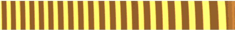
Figure 2.3: Hysteretic image distortion in retrace direction from right to left, \dot{V} < 0 . Scanned is a line pattern with a period of 3.0 \mu\text{m} .
