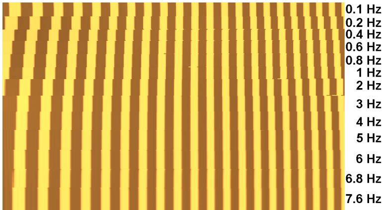
Figure 3.1: Long tube scanner, visualization of time-dependency, 1D3000, table 3.1, trace image. The voltage range is constant at 110 V, the scan frequency has been changed as shown while acquiring the image. It is clearly demonstrated how scan frequency affects the scanned distance.
