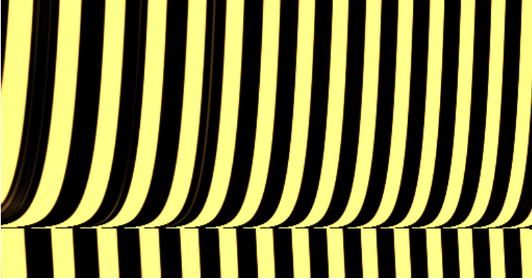
Figure 5.1: Long tube scanner. Sample 1D3000 is scanned upwards at a frequency of 0.1 Hz. At the centre of the image the scan offset was changed from -80 V to 0 V while the SPM continued scanning. The curvature is typically related to "creep" but also contains time-independent transition.
