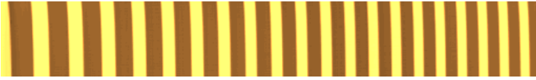
Figure 2.2: Hysteretic image distortion in trace direction from left to right, \dot{V} > 0 . Scanned is a line pattern with a period of 3.0 \mu\text{m} .
