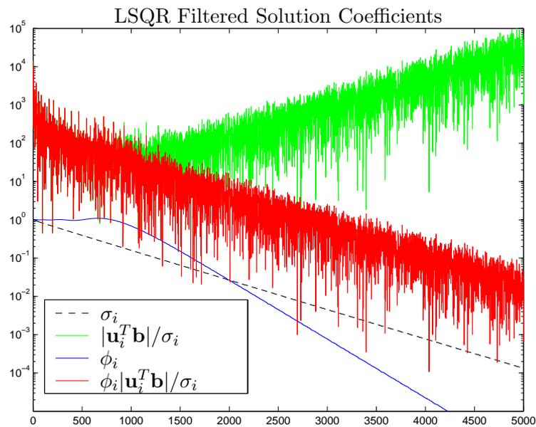
Figure 5.15: Zoom of part of Picard plot for Barbara test problem showing the singular values  $\sigma_i$  as dashed black line, the filter factors as a simple solid blue line, the solution coefficients  $|\mathbf{u}_i^T \mathbf{b}|/\sigma_i$ , that rise in the end caused by the noise entering, in green, and the filtered solution coefficients  $\phi_i |\mathbf{u}_i^T \mathbf{b}|/\sigma_i$  in red. The LSQR filter factors after 10 iterations are used.
