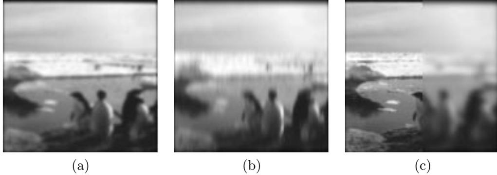
Figure 3.2: Illustration of (a) spatially invariant blur with  $\sigma_c = \sigma_r = 4.5$ , (b) spatially invariant and elliptical blur with  $\sigma_c = 2$  and  $\sigma_r = 10$  (more blurring across rows than across columns), and (c) spatially variant blur as defined in (3.25) with  $\sigma_c = \sigma_r = 2$  in the left side of the image, and  $\sigma_c = \sigma_r = 10$  in the right side of the image.
