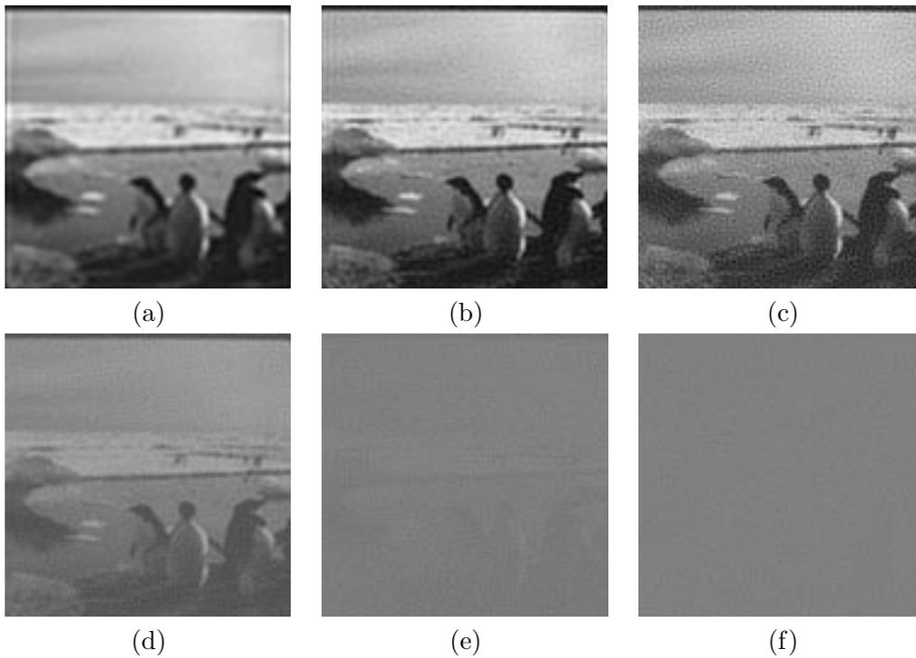
Figure 5.2: *Regularized solutions. (a), (b), and (c) using LSQR after 4, 10 and 25 iterations, and (d), (e), and (f) using GMRES after 4, 10 and 25 iterations.*
