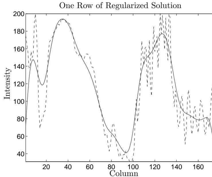
Figure 3.16: One row picked out of the second Tikhonov regularized solution in Fig. 3.15 (h). The dashed line is the true image and the solid line is the regularized solution.
