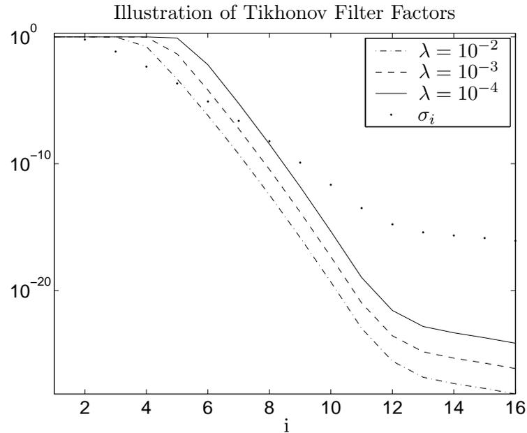
Figure 2.3: Illustration of the Tikhonov filter factors  $\phi_i = \sigma_i^2 / (\sigma_i^2 + \lambda^2)$  for a small test problem. The value of  $\lambda$  is seen to change the cut off in the filter factors, so that lower  $\lambda$  gives a higher cut off point.
