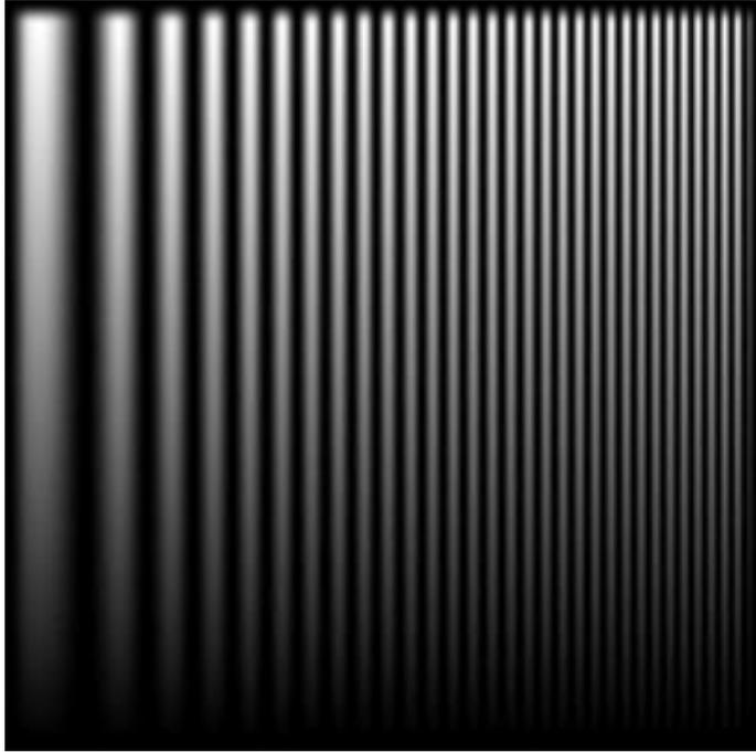
Figure B.6: *Frequency and Amplitude Sweep* – Size  $256 \times 256$  pixels. This image is generated by a MATLAB function found at my homepage <http://www.imm.dtu.dk/~tkj>. The image is always square, and the size is variable from  $32 \times 32$  and larger.
