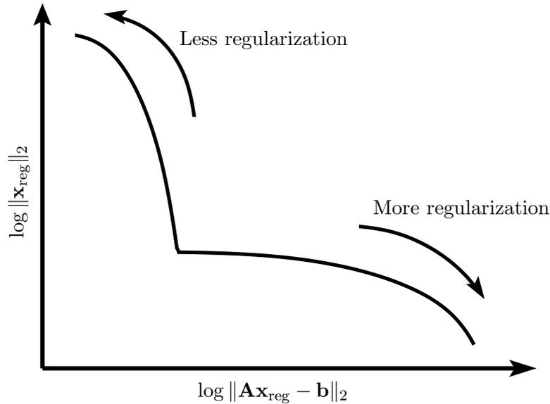
Figure 6.1: *Generic L-Curve showing the theoretical corner arising in the transition from a fast decrease of the residual to a fast increase of the solution norm.*
