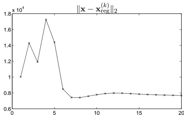
Figure 6.3: Plot showing  $\|\mathbf{x} - \mathbf{x}_{\text{reg}}^{(k)}\|_2$  for the GMRES solution with inner Tikhonov regularization, using the GCV function to choose the regularization parameter.
