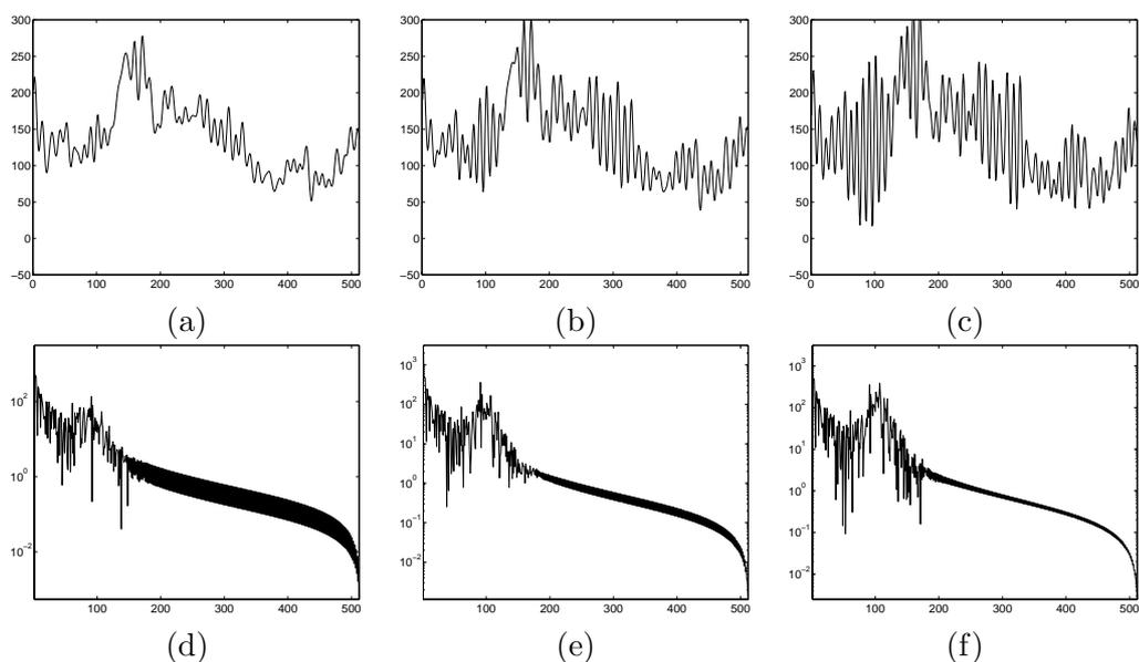
Figure 5.11: (a), (b), and (c) show LSQR regularized solutions to the one-dimensional problem after 10, 20 and 30 iterations. (d), (e), and (f) show the DCT transformed frequency domain of the solutions.
