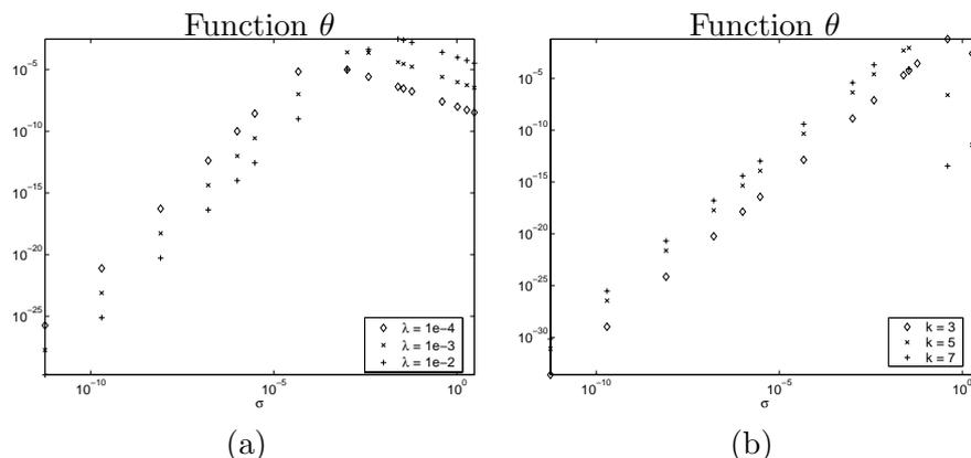
Figure 7.6: (a) Function  $\theta$  plotted using Tikhonov filter factors with different  $\lambda$ . (b) Function  $\theta$  plotted using the filter factors coming from different iterations of the LSQR algorithm. The filter factors are calculated by means of (4.35).
