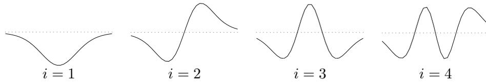
Figure 2.1: First four left singular vectors  $\mathbf{u}_i$ ,  $i = 1, 2, 3, 4$  showing the increasing number of zero crossings, i.e. the increase in frequency.
