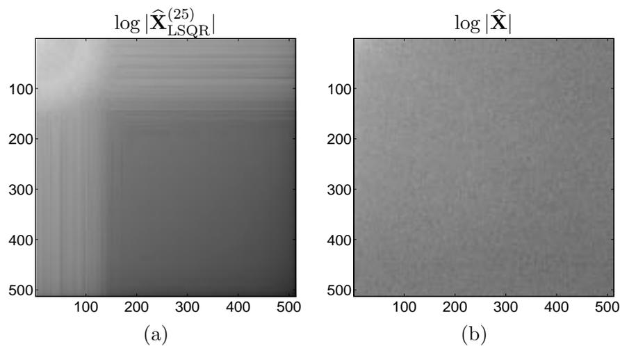
Figure 5.6: (a) Image showing the LSQR solution in Fig. 5.2 (c) transformed to the DCT frequency domain. (b) Image showing the frequency domain of the true penguin image from Fig. B.3.
