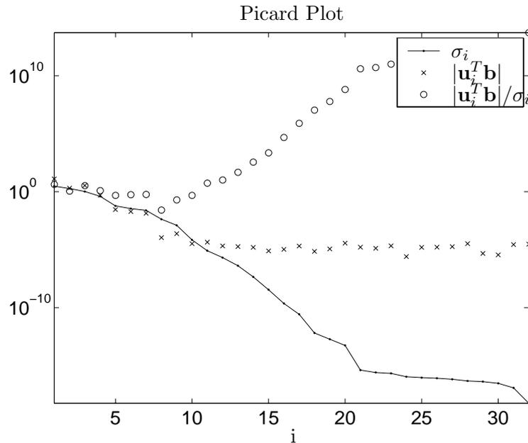
Figure 2.2: Picard plot for simple shaw test problem, showing singular values  $\sigma_i$ , solution coefficients  $|\mathbf{u}_i^T \mathbf{b}|$ , and the ratio between them. The noise level is set to  $\eta = 10^{-1}$ .
