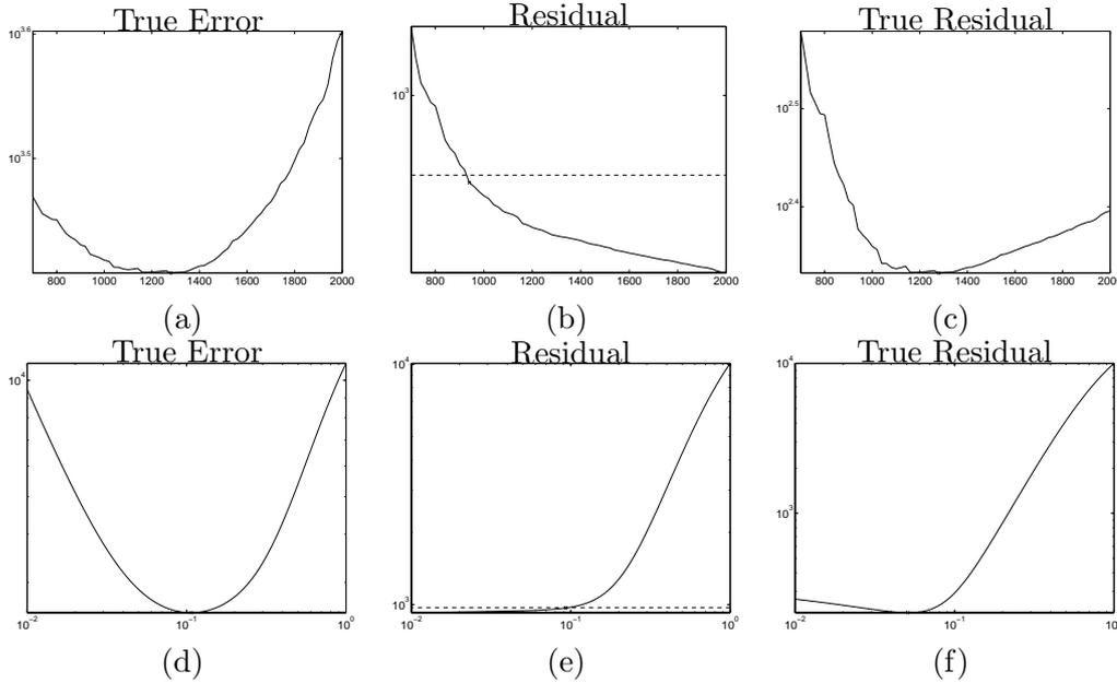
Figure 3.17: (a) Shows the true error  $\|\mathbf{x} - \mathbf{x}_{\text{reg}}\|_2$ , (b) shows the residual  $\|\mathbf{Ax}_{\text{reg}} - \mathbf{b}\|_2$  and with dashed line the size of the noise  $\delta_e$ , and (c) shows the true residual  $\|\mathbf{Ax}_{\text{reg}} - \bar{\mathbf{b}}\|_2$ . All for the TSVD solutions, including a varying number of singular components. (d), (e), and (f) show the same information for the Tikhonov solutions with varying  $\lambda$ .
