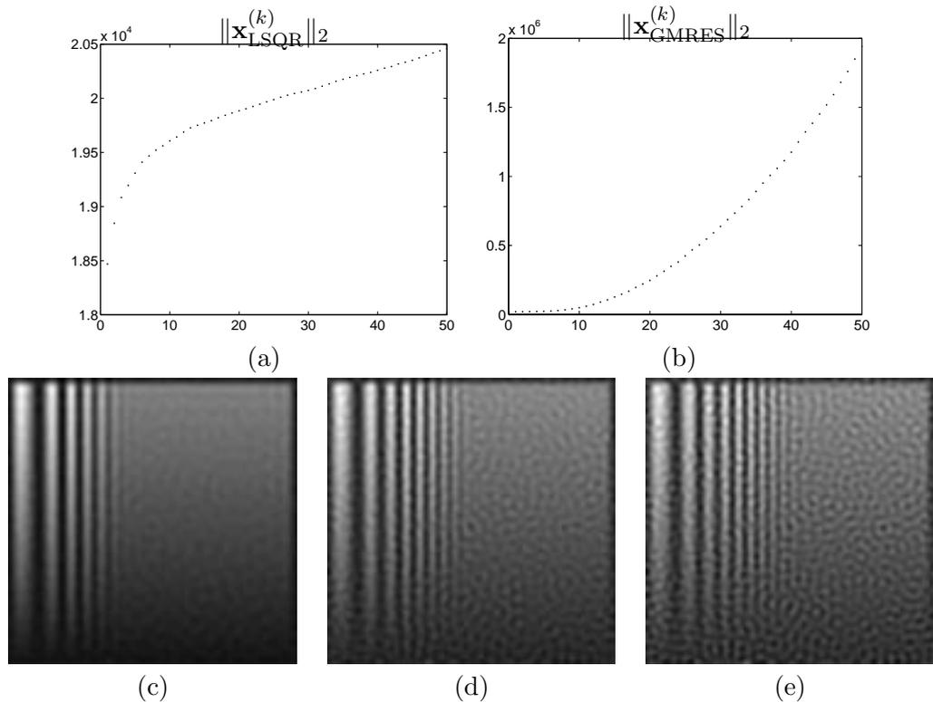
Figure 7.3: Two-norm of the solutions for (a) LSQR and (b) GMRES over 50 iterations. (d), (e), and (f) show the LSQR solution after 10, 30 and 50 iterations.
