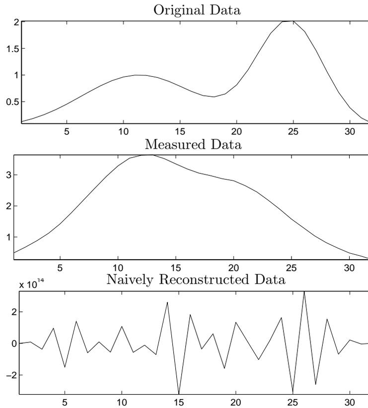
Figure 1.2: Example showing a one-dimensional function, a blurred measurement of the function, and a naive reconstruction.
