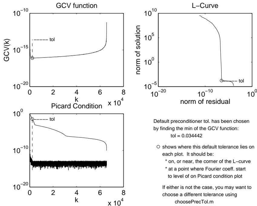
Figure 6.5: Illustration of the truncation parameter  $\tau$  found for preconditioner to the Satellite example.
