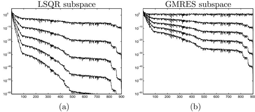
Figure 5.3: First five Krylov vectors in the symmetric case for (a) LSQR,  $\Sigma^{2k-1}\mathbf{U}^T\mathbf{b}$  and (b) GMRES,  $\Sigma^{k-1}\mathbf{V}^T\mathbf{b}$  for  $k = 1, \dots, 5$ . The ones in the top are the first vectors,  $\Sigma\mathbf{U}^T\mathbf{b}$  and  $\mathbf{V}^T\mathbf{b}$ , respectively.
