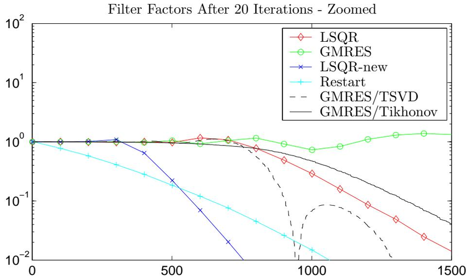
Figure 6.12: Zoom of first part of the filter factors. Showing that GMRES with inner Tikhonov regularization has almost no oscillations.
