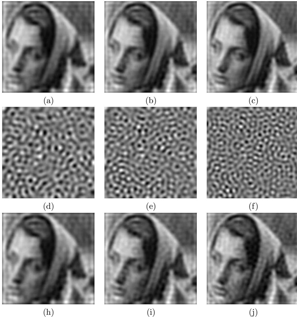
Figure 3.13: Images (a), (b), and (c) show the TSVD solutions to the true blurred right-hand side  $\tilde{\mathbf{b}}$  for 800, 1000, and 1200 included SVD components; (d), (e), and (f) show the TSVD solutions to the noise vector  $\mathbf{e}$ ; and (h), (i), and (j) show the TSVD solutions to the blurred and noisy right-hand side  $\mathbf{b}$ .
