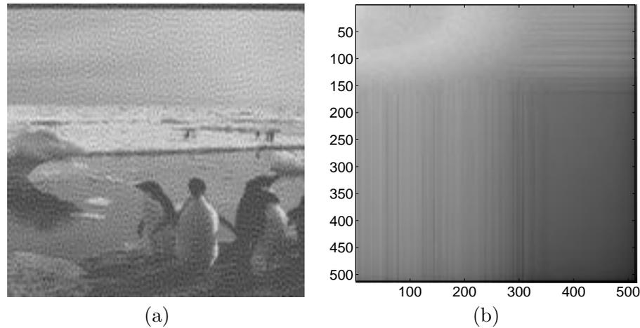
Figure 5.8: (a) LSQR solution of penguin image non-symmetrically blurred after 25 iterations, and (b) the frequency representation of the regularized solution.
