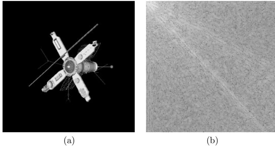
Figure 3.1: Illustration of two-dimensional DCT. (a) Is the original test image  $\mathbf{X}$ , and (b) is a visualization of the 2D-DCT of  $\mathbf{X}$ ,  $\log|\hat{\mathbf{X}}|$ . The logarithm is used while the low frequencies in the upper left corner are much more intense than the higher frequencies, and most of the image would have been black if the logarithms was not used.
