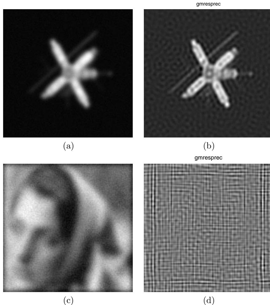
Figure 6.4: (a) Shows a blurred artificial satellite and (b) is the preconditioned GMRES solution after only one iteration. (c) and (d) show the similar test for the Barbara image, used earlier.
