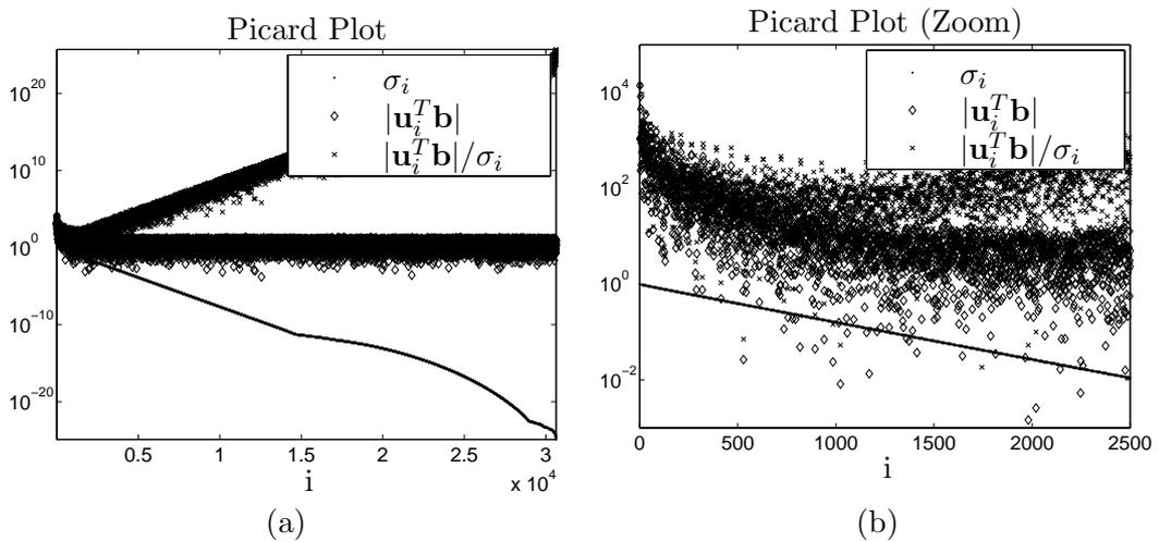
Figure 3.12: *Illustration of Picard plot for an image problem. In (a), the full plot is shown, and in (b), the interesting part is zoomed up.*
