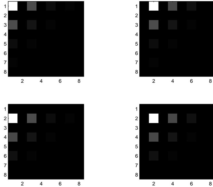
Figure 3.3: 2D-Plot of first four DCT-transformed right singular vectors. First singular vector is at top right, the next top left, the third at bottom right and the fourth at bottom left.
