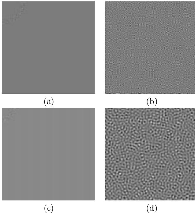
Figure 5.7: (a) Artificially generated band of normal distributed random values to emulate band in frequency domain.  $f_1 = 0.20$  and  $f_2 = 0.25$  (b) The spatial representation of the band of random intensities in the frequency domain. (c) Frequency domain with  $f_1 = 0.10$  and  $f_2 = 0.15$ . (d) Spatial representation of (c).
