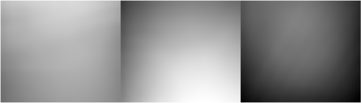
Figure 3.15 R, G and B Color Shading with Cosmimar 25 mm lens and JVC KY-55 3xCCD
