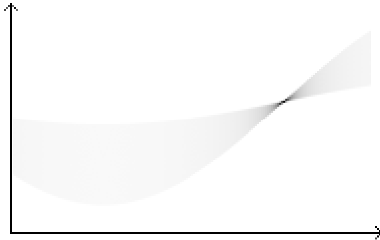
Figure 4.25 The Hough parameter space of a single 45 deg angle line. The quantization is 180x180.
