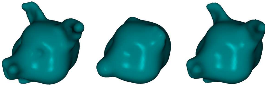
Figure 7.12: Volume Sculpture of a “marzipan pig”. Normal (left). After open with a sphere of radius 3 (centre) and after close with the same sphere (right).
