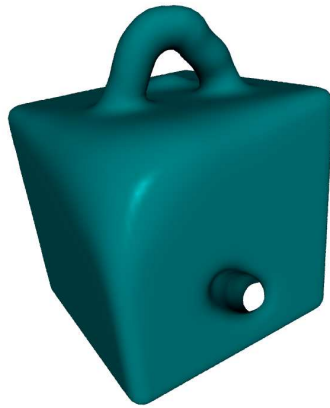
Figure 7.8: Add blob and remove blob have been used to create new features on a cube solid.
