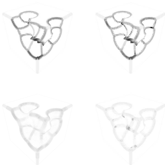
Figure 6.14: Visualization of gradient magnitude error. min CSG (top left,) FMM CSG (top right), smoothed FMM CSG (bottom left), morphological approach (bottom right). White denotes a gradient length error of 0 whereas black denotes a gradient length error of 1.
