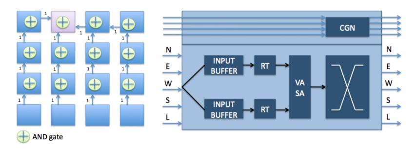
The GCN consists of a one-bit wide subnetwork per node, each collecting the ACKs from all other nodes
