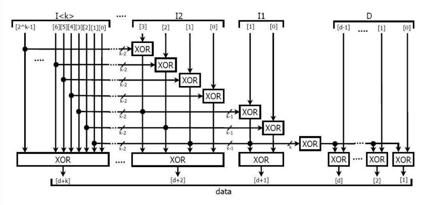
The hardware for a particular M-of-N1 code can be reused for any M-of-N2 code where N2 < N1, if the extra inputs in the inversion field are not used.
