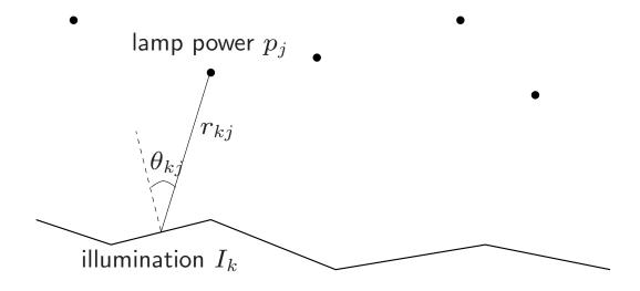
intensity  $I_k$  at patch k depends linearly on lamp powers  $p_j$ :  $I_k = a_k^T p$
