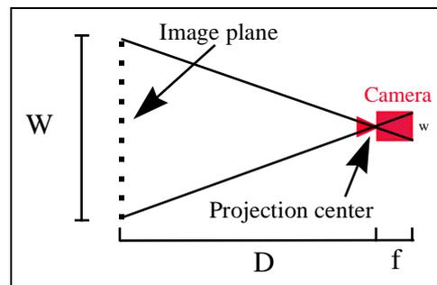
Fig 2-1. The Pinhole model
