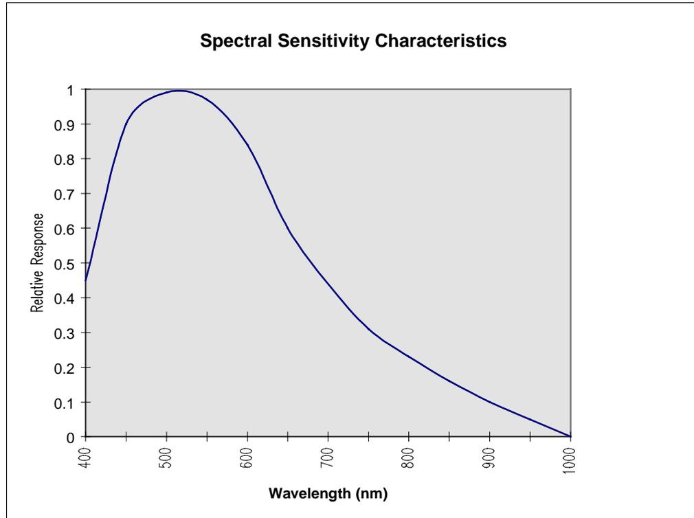
Fig 5-5 Spectral Sensitivity Characteristics for Sony CCD chip.
