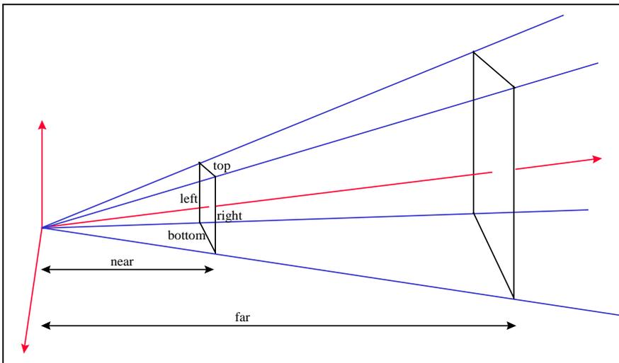
Fig 3-1 The perspective viewing volume specified by `glFrustum`
