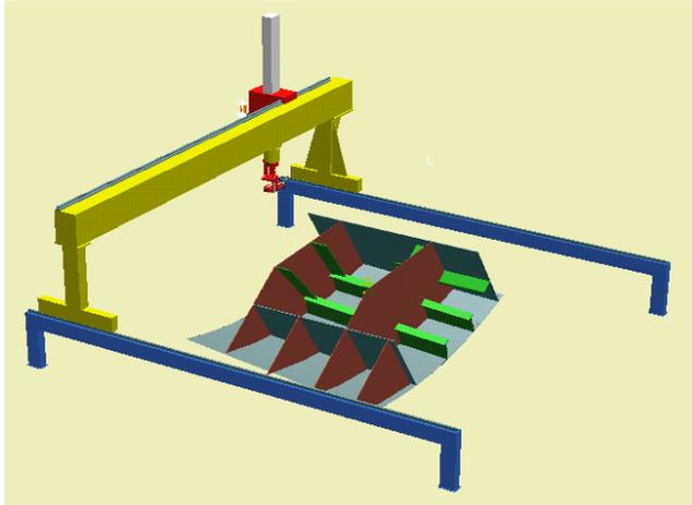
Fig 3-5 The 11 axes robot manipulator
