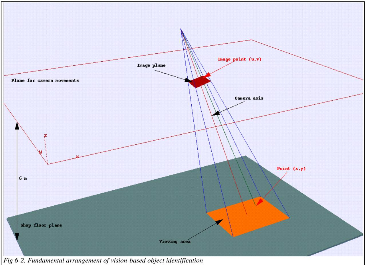
Fig 6-2. Fundamental arrangement of vision-based object identification
