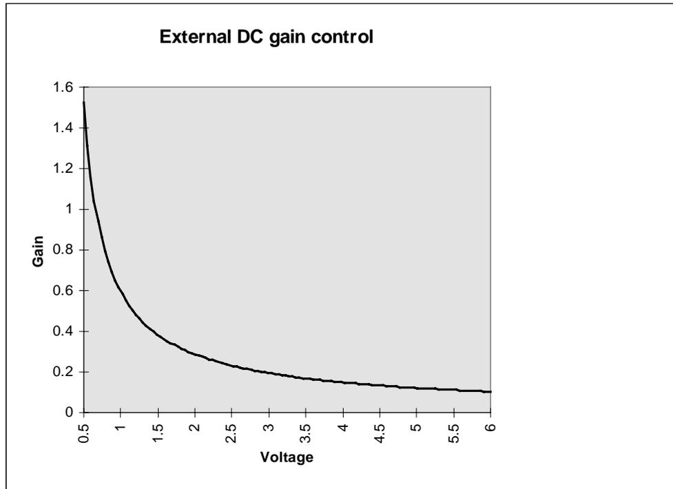
Fig 5-4 Amplification of video signal as a function of an external DC voltage.
