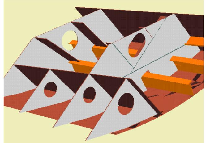
Fig 3-6 CAD model of mock-up
