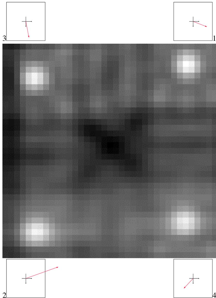
Fig 4-20 Illustration of how the centre of the templates is shifted with subpixel accuracy. The boxes surrounding the image illustrate one pixel and the red arrow shows how much the centre should be shifted (see also Table 4.1)
