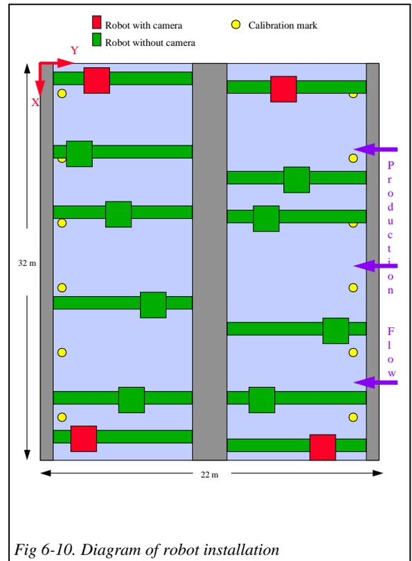
Fig 6-10. Diagram of robot installation
