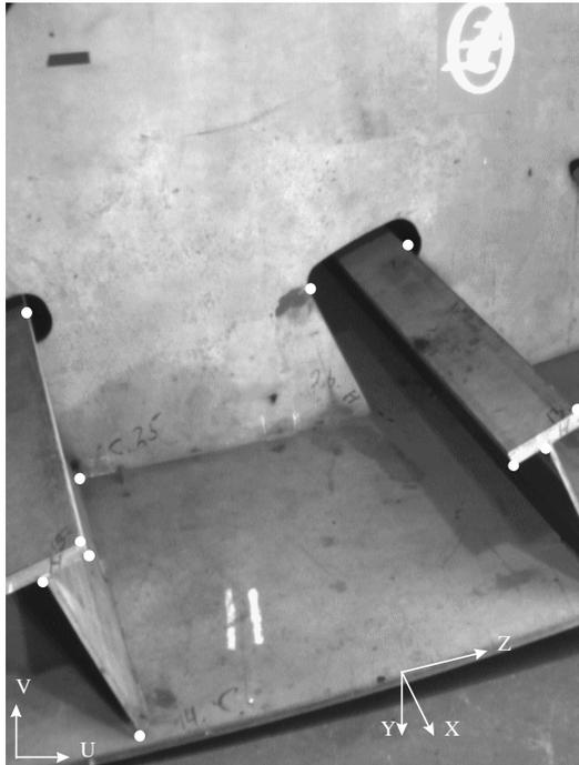
Fig 3-8 Selected image with identified calibration points
