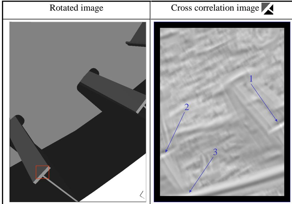
Fig 3-20 Rotated virtual image & cross correlation image (obtained with optimal feature rotation).
