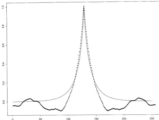
Fig 4-10 Analytical function and slice through autocorrelated image..
