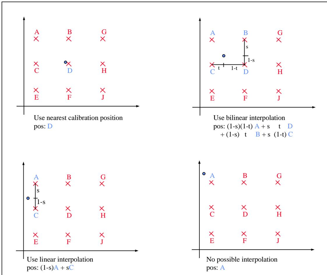
Fig 6-15. Examples of how to use the calibration grid
