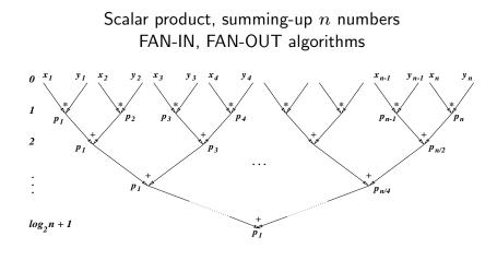
Binary tree algorithm represented by a cascade graph to compute  $\sum_{i=1}^n x_i y_i$ , where  $n=2^s(s=3)$
