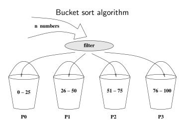
Quick sort in each bucket - serial complexity to sort k numbers:  $O(k \log k)$
