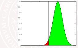
If the number of bit error exceeds the specified error coding threshold, the packet is lost
