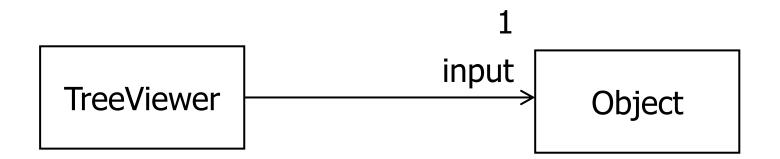
Shows the input as a tree (with all the features of a tree view like opening and closing sub-trees, etc)
