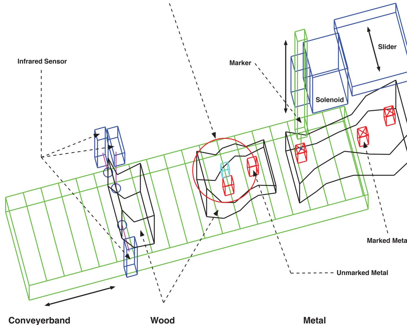
A simple conveyerband used to move the pieces of wood through the different stages of the system.
