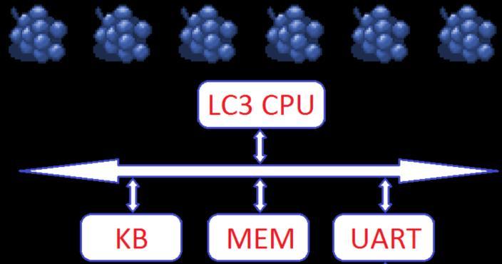
In this project we have been using an LC3 computer system which is simulated on a Nexys 3 FPGA board. The FPGA board is connected to a PC through a serial connection. The game logic (a C program) then transmits information about how elements should be drawn on the screen to the PC, which then takes care of rendering the game.
