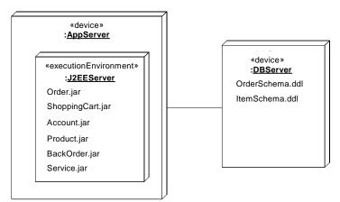
Figure 10.14 - Notation for a Device
