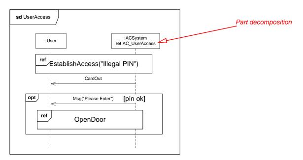
Figure 14.20 - Part Decomposition - the decomposed part
