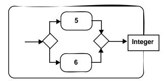
Figure 12.136 - Example ValueSpecificationAction
