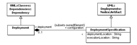
Figure 10.5 - Metaclasses that define component Deployment
