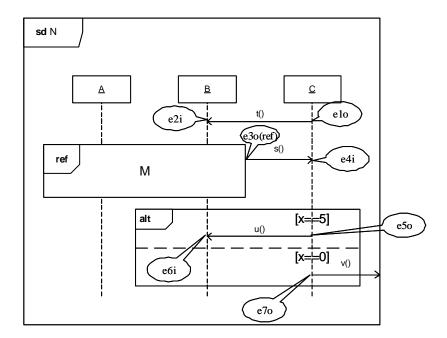
Figure E.1 - Sequence diagram enhanced with identification of the Event occurrences
