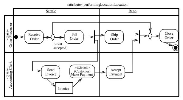
Figure 12.61 - Activity partition using multidimensional swimlane example
