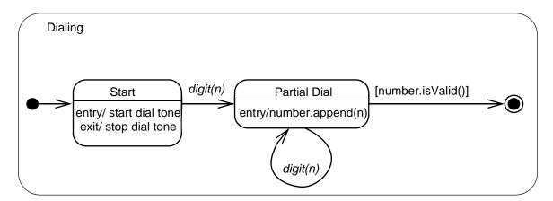
Figure 15.33 - Composite state with two states
