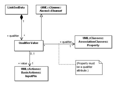
Figure 11.14 - Link identification (CompleteActions)
