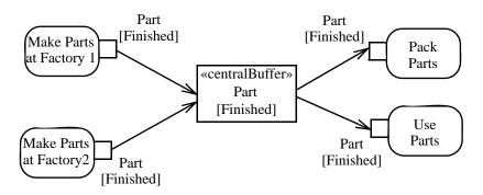
Figure 12.69 - Central buffer node example
