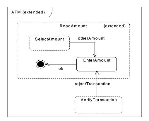
Figure 15.43 - An extended state machine
