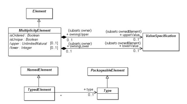
Figure 7.5 - Multiplicities diagram of the Kernel package
