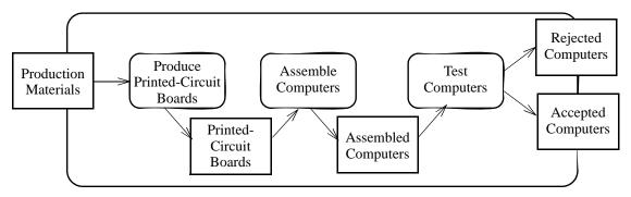
Figure 12.55 - Example of activity parameters.nodes
