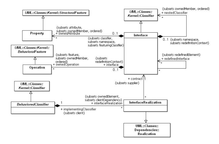
Figure 7.16 - Contents of Interfaces package
