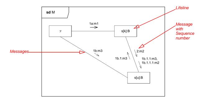
Figure 14.27 - Communication diagram
