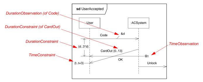
Figure 13.15 - DurationConstraint and other time-related concepts
