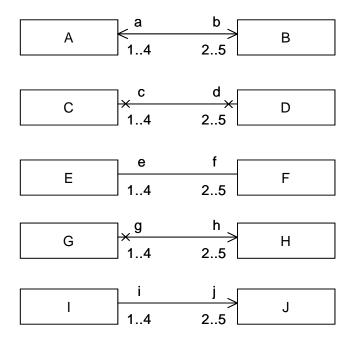
Figure 7.23 - Examples of navigable ends
