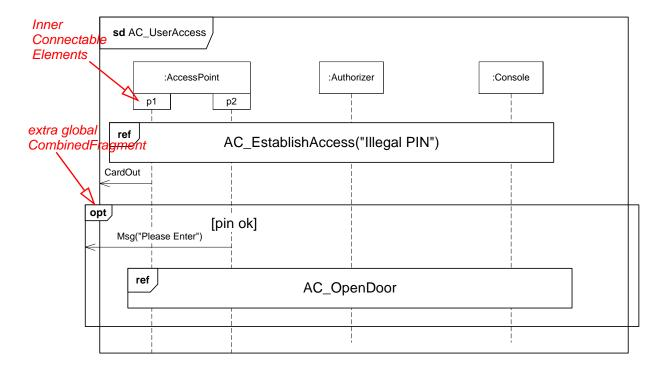
Figure 14.21 - PartDecomposition - the decomposition
