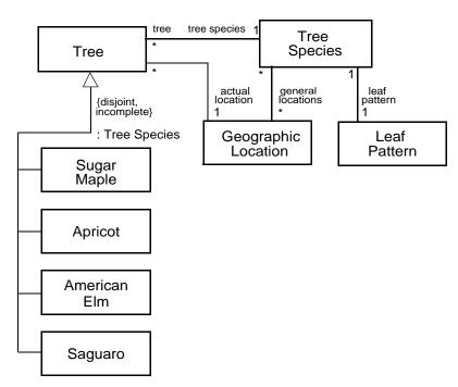
Figure 7.49 - Power type example and notation
