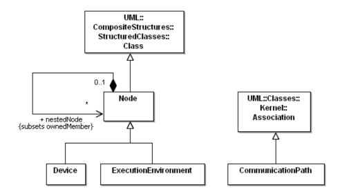
Figure 10.3 - The definition of the Node concept
