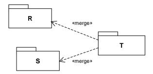
Figure 7.70 - Introducing additional package merges
