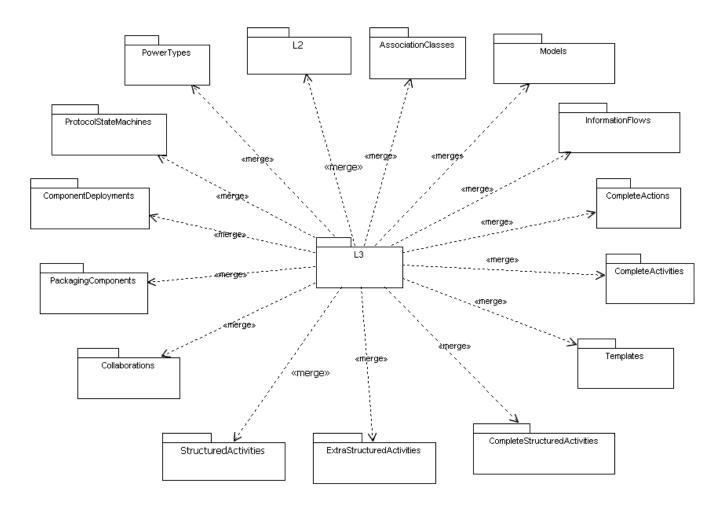
Figure 2.4 - Level 3 top-level package merges
