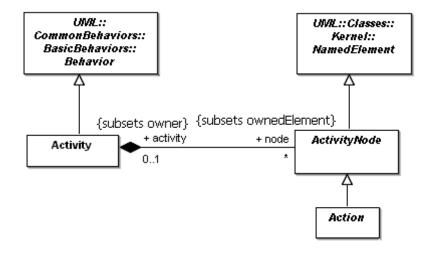
Figure 12.2 - Fundamental nodes
