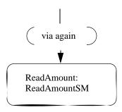
Figure 15.9 - Alternative Entry Point notation
