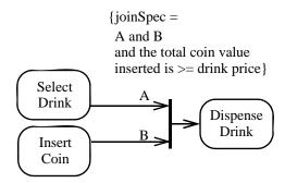
Figure 12.104 - Join node example
