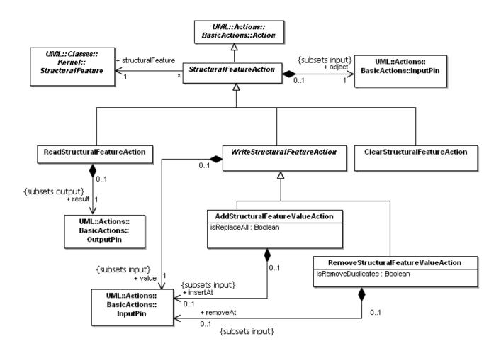
Figure 11.7 - Structural Feature Actions
