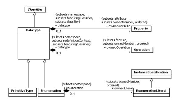
Figure 7.13 - DataTypes diagram of the Kernel package
