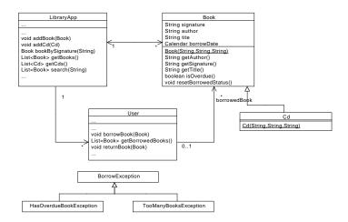
The class diagram after refactoring
