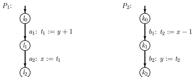
Let the global state be given by a vector  $(x, y, t_1, t_2, \pi_1, \pi_2)$  where  $\pi_i$  is the control pointer for process  $P_i$ . Assuming arbitrarily  $t_1$  and  $t_2$  to be initially 0, the transition system for the concurrent systems is given by the transition graph:
