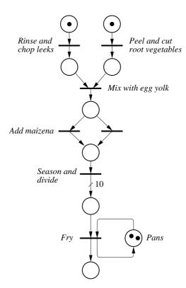
Remarks: Whether to add maizena or not is represented by a choice with a void branch. The the crossed arc with a 10 represents 10 arrows corresponding to the division into portions. According to the way we define simultaneous firings of a transition with itself, the last part allows for frying two pancakes at a time.
