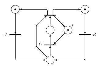
[Note how C is prohibited in firing twice by the place (\*) corresponding to control of  $P_3$ ]
