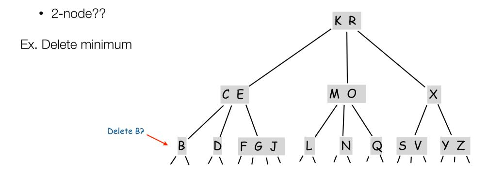
Idea: On the way down maintain the invariant that current node is not a 2-node.
