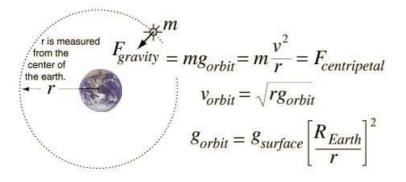
Figure 1: The orbit of a satellite
